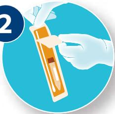
Open the swab container and remove the swab, taking care not to touch the tip to any surface or lay it down.
